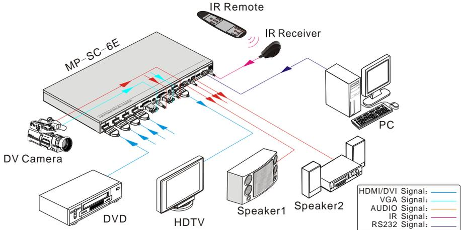
Figure 3- 1 Connection Diagram
